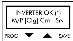
This occurs if the inverter is disabled (IFD SW and VTC SW) or no run command is sent or the frequency reference is equal to zero (IFD SW).
