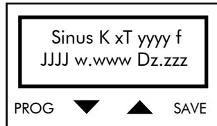
Field JJJJ relates to the application SW programmed (IFD SW or VTC SW).
