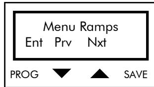
Press PROG (Ent) to access the first page of the Ramps submenu. Press ↑ (Nxt) and ↓ (Prv) to scroll through the submenus.
