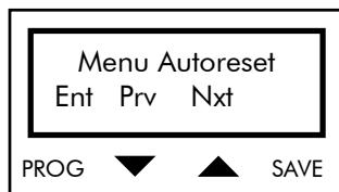
Press PROG (Ent) to access the first page of the Autoreset submenu. Press ↑ (Nxt) and ↓ (Prv) to scroll through the submenus.
