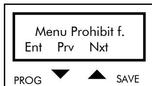
Press PROG (Ent) to access the first page of the Prohibit Frequencies submenu. Press ↑ (Nxt) and ↓ (Prv) to scroll through the submenus.
