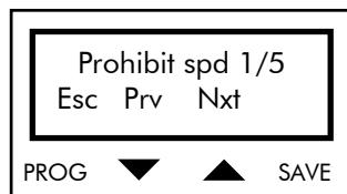
Press PROG (Esc) to return to the Prohibit Speeds submenu access page. Press ↑ (Nxt) and ↓ (Prv) to scroll through the parameters.
